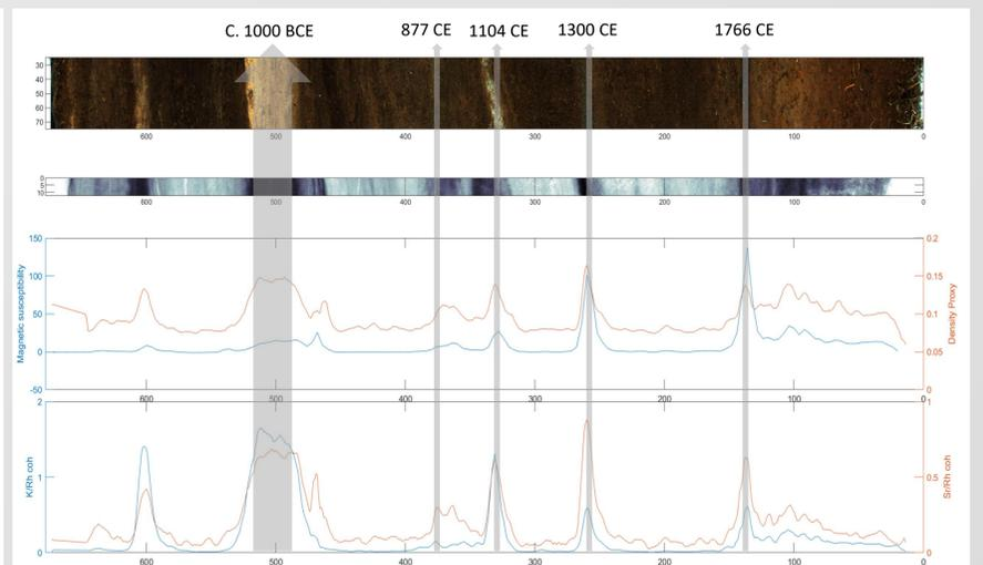
Figure 6. Kot. Results from XRF scanning and magnetic susceptibility measurement. Also shown are ages of the tephra layers within the peat. Depth measurements are in mm. Values are arbitrary.
