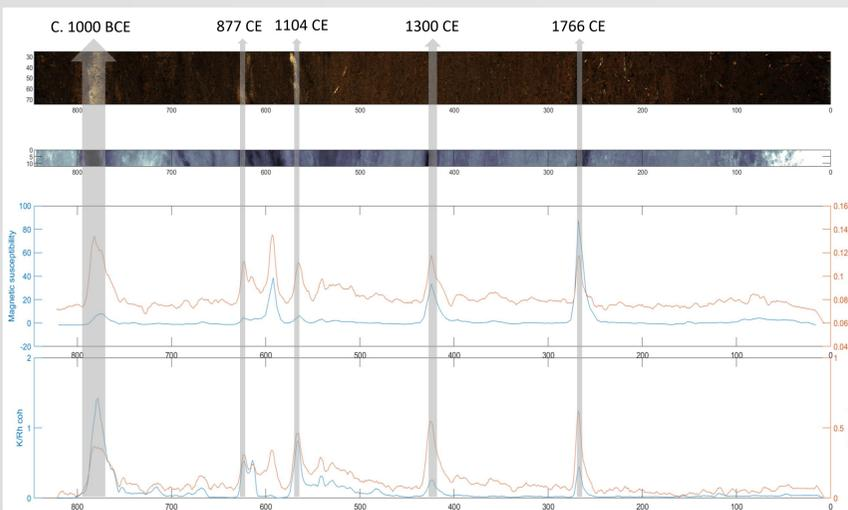
Figure 5. Tunga. Results from XRF scanning and magnetic susceptibility measurement. Also shown are ages of the tephra layers within the peat. Depth measurements are in mm. Values are arbitrary.
